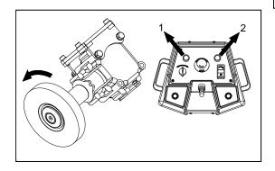
**9 – ROTATION OF THE BRUSH** — Do Press Button No(1) which is showed on figure to rotate the brush , Do Press Button No(2) which is showed on the figure to stop the brush .
