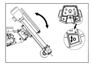
6 – MAIN SUPPORT BODY — Do push the joy stick which is showed on the figure to the right and left to make turning of movement of Support body
