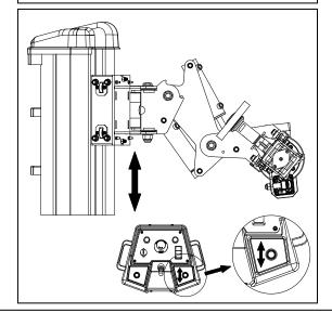
**5 – VERTICAL CRADLE BODY GROUP** — Do Push the joy stick which is showed on the figure to down and up to make move Vertical Cradle Body to down and up.
