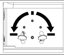
**BALANCER GROUP** During the Rim Tightening operation It provides the rim to center the mirror easily and makes clamps clutch the rim
