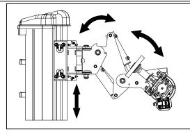
**CRADLE AND SUPPORT GROUP** During the Rim Polishing It provides to touch the brush easily whole surface of the rim.
